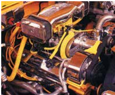
High thermal and chemical resistance and wide color/size selection make Flexo PET ideal for customizing and protecting the wires, hoses, and cables in custom and classic cars.
